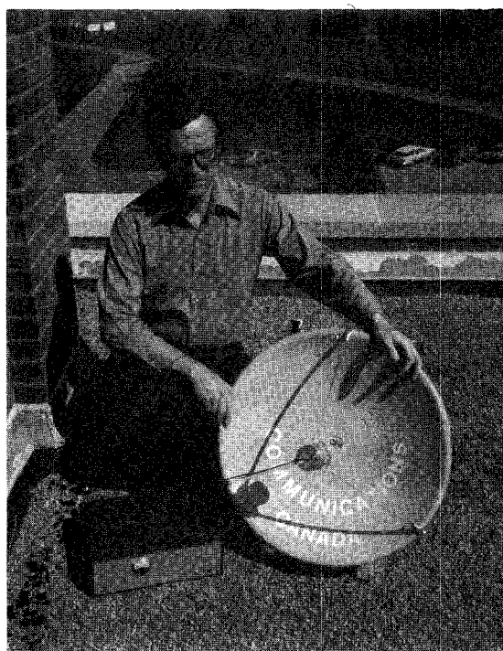
Fig. 11. The complete low-cost earth terminal using the 0.6-m reflector with the 90° scalar feed outdoor unit. The indoor unit is also visible at the left.
